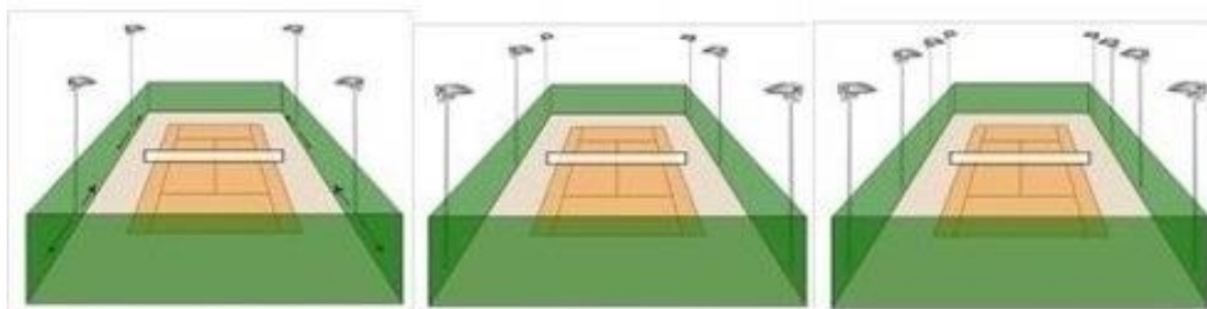
Figure 2. Typical mast layout for outdoor courts.
